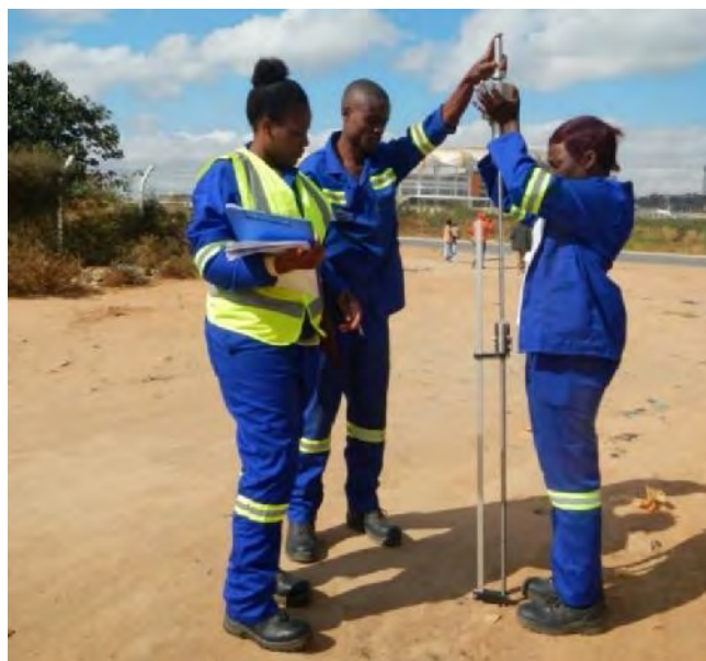
Figure 4-1: Team of three persons required for DCP testing
