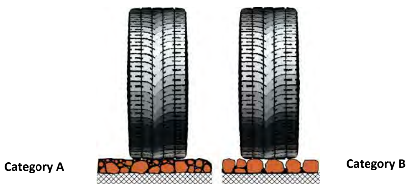
Figure 11-3: Different performance mechanisms of bituminous surfacings
