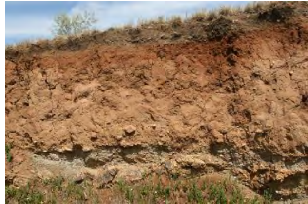
Figure 5-2: Typical deposit of transported sandy material
