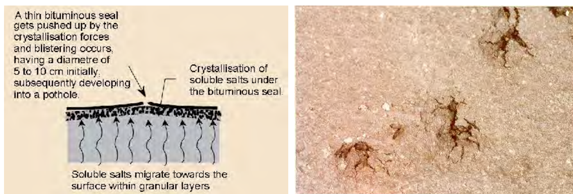
Figure 4-15: Mechanism of salt damage
