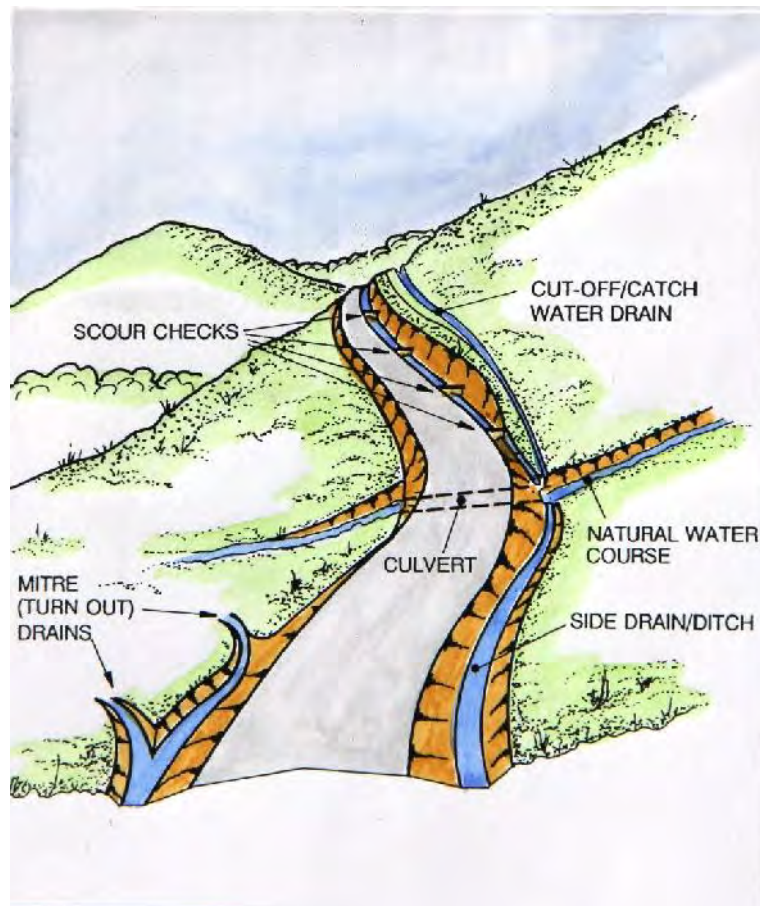
Figure 3: Main drainage elements
