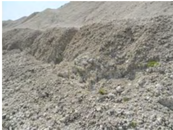
Figure 5-4: Typical appearance of nodular calcrete deposit
