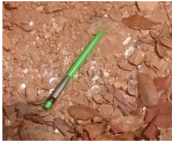
Figure 4-18: Micaceous soil with large flakes of mica
