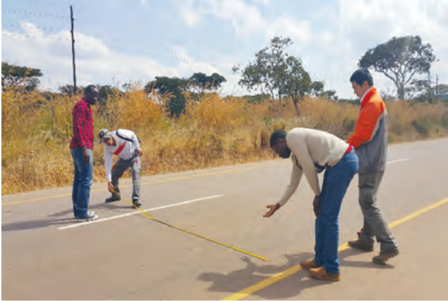
Figure 9: Pavement width measurement
