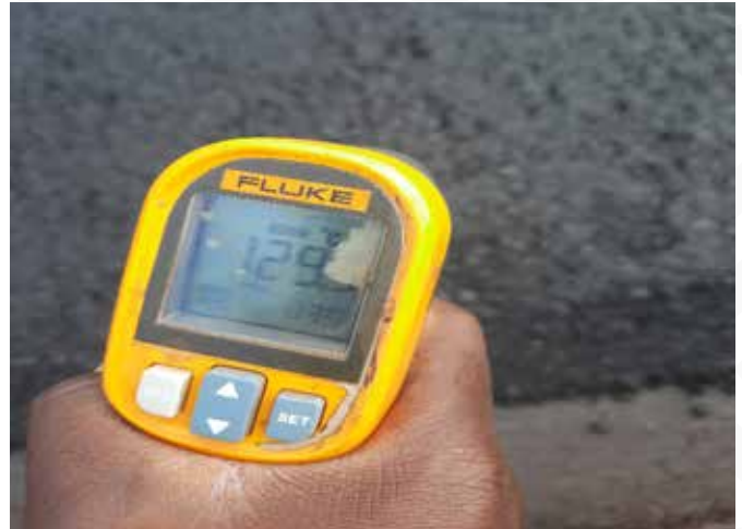
Figure 25: The RDA team checking whether the asphalt concrete surfacing on the Chinsali to Nakonde Road Lot 1 is of the right temperature as part of quality control and assurance during the vendor rating inspections
