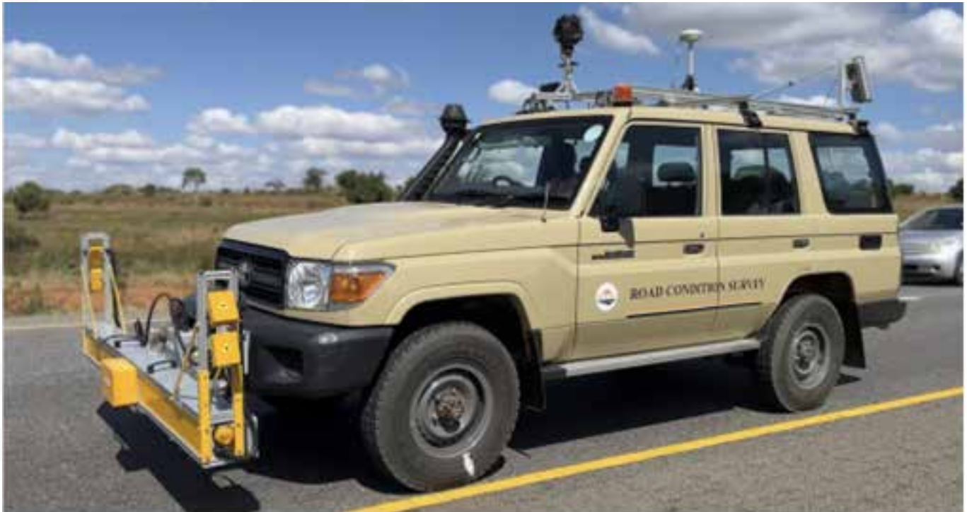
Figure 4: Road Condition Survey Vehicle
